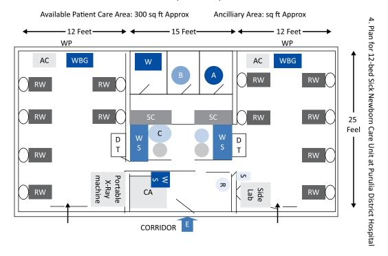
Legends: A: Autoclave, AC: Split Air conditioner, B: Washing Machine, C: Computer, CA: Changing area, DT: Drugs Trolley, E: Main Entrance, R: Refrigerator, RW: Radiant Warmer, SC: Storage cabinet, W: Weghing scale, WB: Wash Basin WP: Window, WS: Work station, Viewing window: ← Doctors' office cum Teaching Room and Step-Down units are located on opposite side of the corridor.
